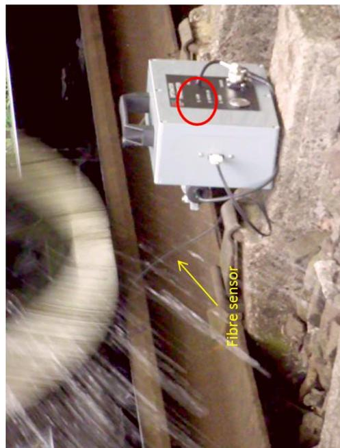
Optonator Transmitter – just before and just after the leading wheel enters the Track Worker Safety zone
