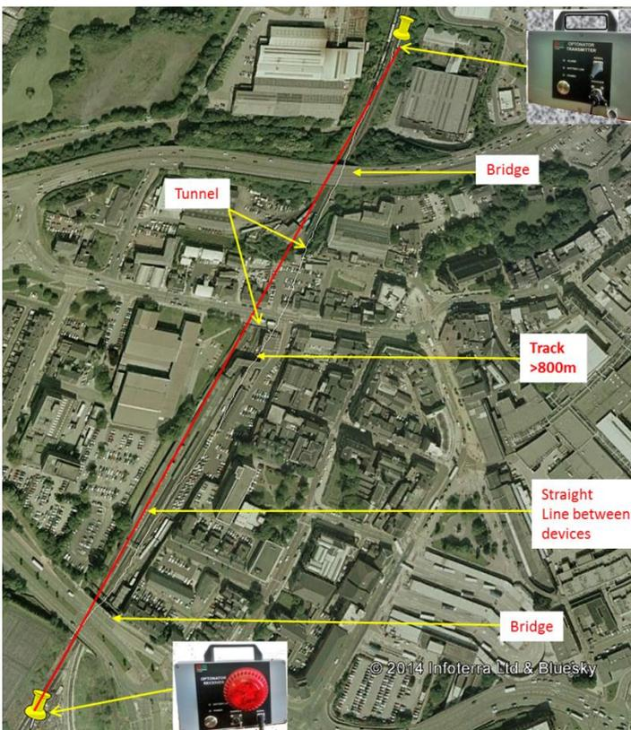
Trialling: 800m track length, which included the effects of a tunnel, 2 bridges, across station platform and vehicle stabling, a curved track structure, and in a town centre environment with various interference .
